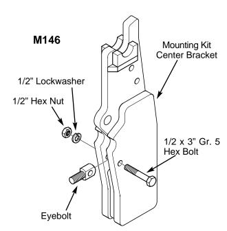
Verify that all mounting kit hardware has been torqued as specified before installing loader.
